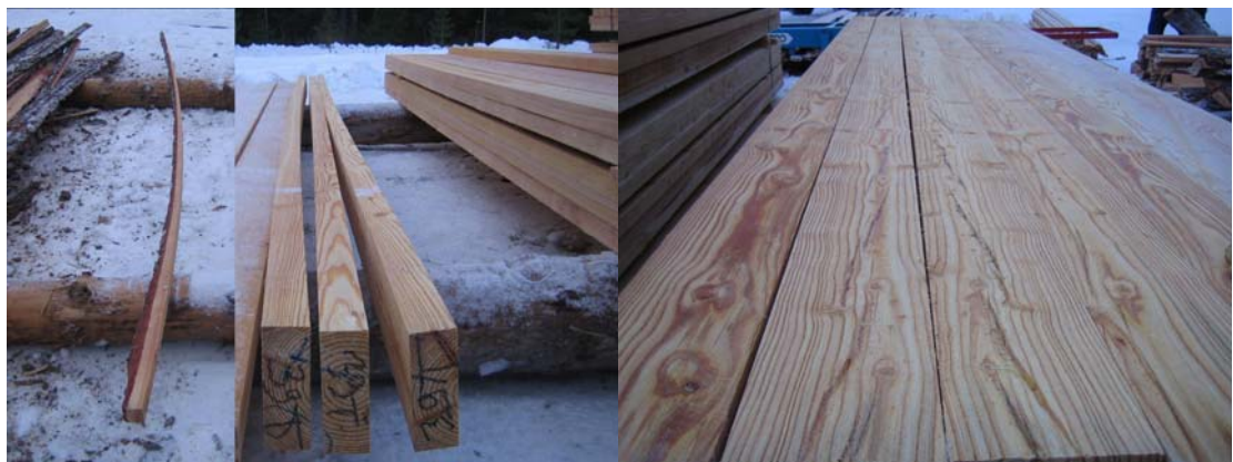
FIGURE 3. Relieved growth tensions in the strips and planks after sawing (left and middle). Large resin pockets in the planks from near the pith (right)
